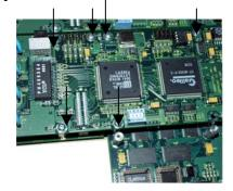
firmly. Figure 3.6.3a: Top View - 6 retaining s crews shown by arrows
